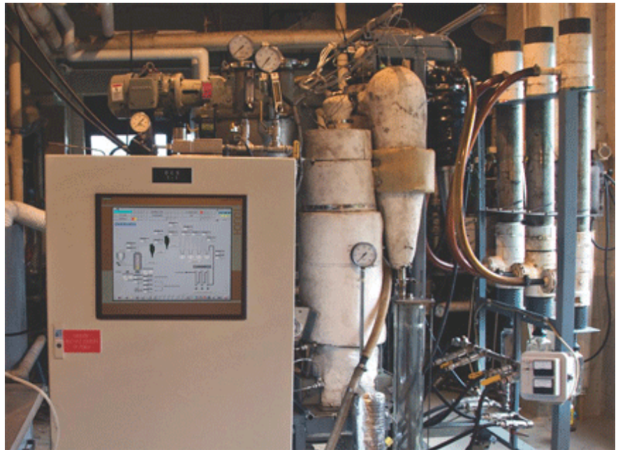
Pyrolysis reactor used by research scientists at the Agricultural Research Service, Eastern Regional Research Center in Wyndmoor, PA
